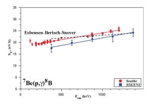
**FIGURE 2.** Extracted  $S_{17}$  from the RIKEN2 CD data [3] using first order electric dipole interaction as shown in [5], compared to the DC capture data published by the Seattle group [10] and the so called reconciled slope calculated by EBS [9]. The shown RIKEN2 data include systematic uncertainties (equal or slightly smaller) as published [3].
