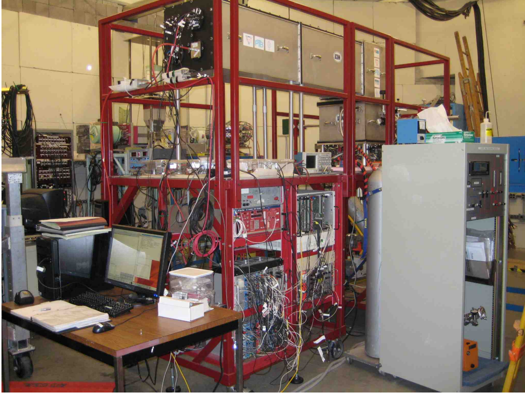
Figure 10. A photograph (back view) of the O-TPC setup placed on a movable platform in the beam line at HIγS. The beam enters the TPC from the front and the source is inserted from the back. Shown are the gas handling system (back right), TPC, mirror box, optical readout box, CAEN high-voltage power supply, electronics and VME DAQ system.
