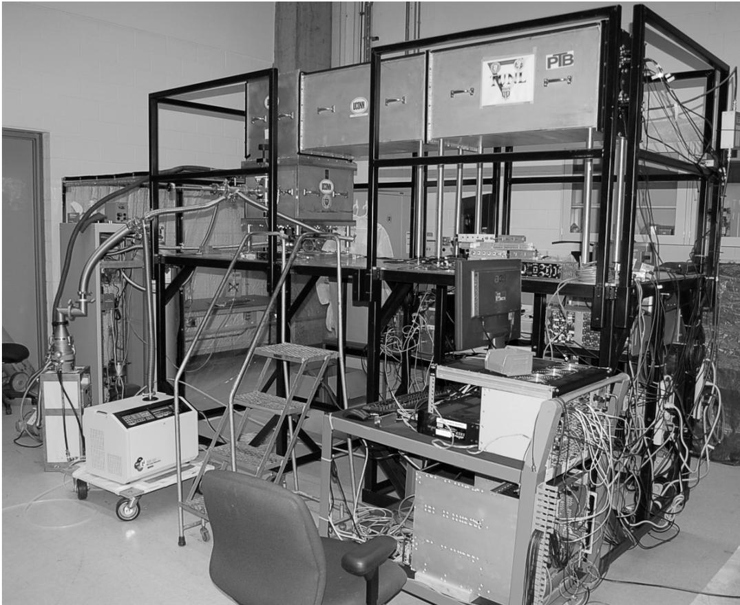
Fig. 6.1: The O-TPC mounted to the frame built at UConn with the data acquisition system (lower right) and gas handling system with leak detector (left).
