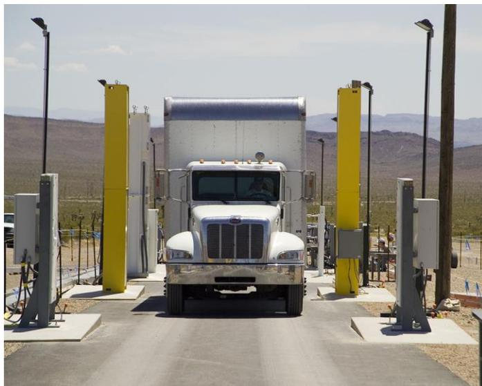
Figure 1.15: A truck going through a portal monitor [31].
