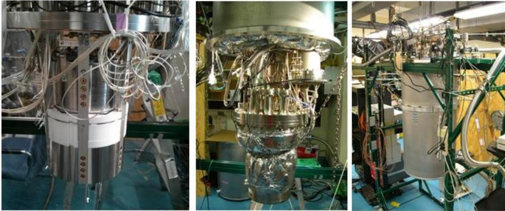
Figure 2.5: “Russian doll” images of PIXeY. Left image: inner detector showing top PMT block, bottom PMT block, and field region. Middle: Stainless steel outer can which forms fits around the inner region, in order to keep the amount of liquid xenon used to a minimum. Right: Outermost can which insulates the inner can. The operational temperature of the detector is 175K, which liquefies the xenon.
