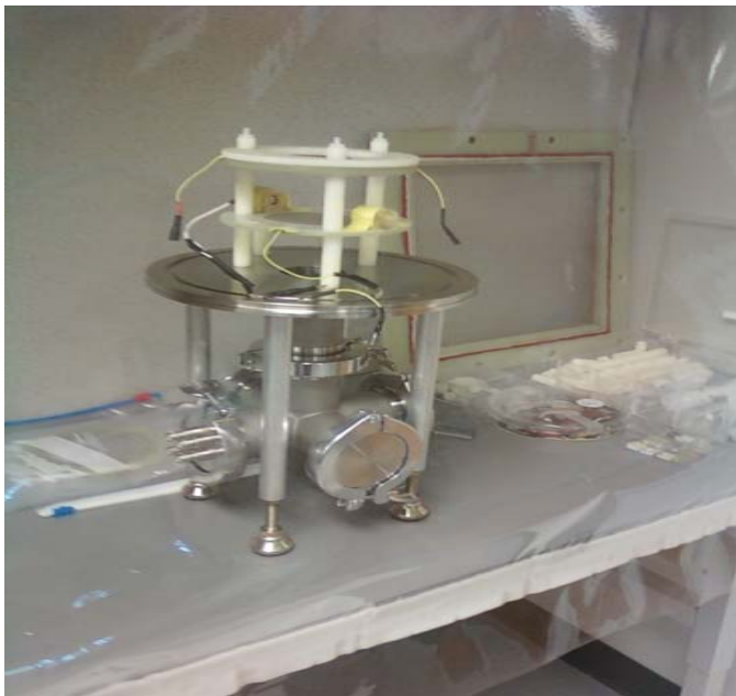
Fig. 1: The drift volume and multiplication grids of the OPAC2 detector together with a test alpha-source and trigger silicon detector.
