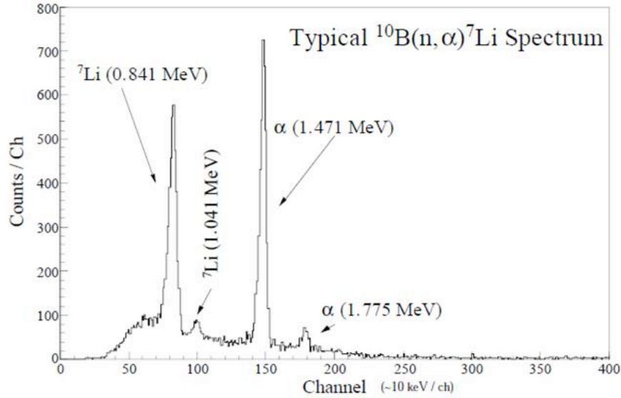
*Fig. 5: A typical  $^{10}\text{B}(n, \alpha)^7\text{Li}$  single's spectrum measured at Yale with a similar type of arrangement of Si detectors [17].*
