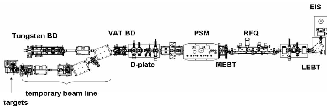
*Fig. 3: Layout of SARAF Phase I and the temporary beam line.*
